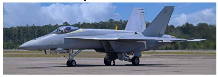
Boeing's iconic representation of excellence in naval aviation, the Super Hornet test aircraft was recently delivered to the US Navy's Blue Angel flight demonstration squadron. The conversion of F/A-18 Hornets and Super Hornets into Blue Angels is carried out at Boeing's Cecil Field facility in Jacksonville, Florida. Major modifications include the addition of an oil tank for the smoke-generation system, fuel systems that enable the aircraft to fly
