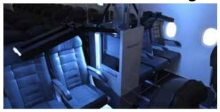
Honeywell and Dimer LIC have entered into a strategic worldwide partnership for bringing the technology of ultraviolet cleaning to airlines. The Honeywell UV Cabin System is roughly the size of a beverage cart and has UVC light arms. These arms spread across the surface and sweep the aircraft cabin in less than 10 minutes. It is proved that if properly applied it can destroy bacteria and virus to a considerable extend.
