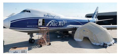
VD Gulf has introduced an inflatable shelter that could be set up very quickly, allowing maintenance on aircraft in adverse weather conditions or when hangar space is not readily available.
