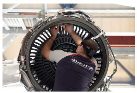
Jet Aviation recently delivered the first fan case modification on a Falcon 7X in Basel. The company has received MRO authorization from Pratt & Whitney to modify fan cases on PW307A and PW307D engines installed on Falcon 7X and Falcon 8X aircraft. It has since
