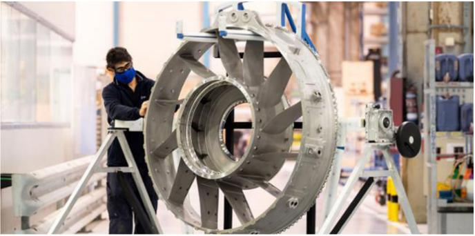
Over the coming weeks, the TBH will be assembled to the UltraFan intermediate pressure turbine, also designed and manufactured by ITP Aero, for final assembly on the complete engine at Rolls-Royce's Derby facilities.
