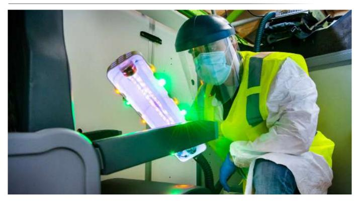
Boeing and Healthe entered into a patent and technology license under which Healthe will manufacture an ultraviolet (UV) wand designed to sanitize airplane interiors. Boeing designed and developed the UV wand as part of the company's Confident Travel Initiative (CTI) to support customers and enhance the safety and well-being of passengers and crews during the COVID-19 pandemic.
