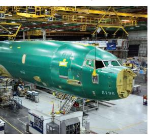
derivative of the Boeing 737 Next-Generation commercial aircraft, the P-8 is first assembled at Boeing Commercial Airplanes' 737 production line, where the fuselage receives additional wiring and systems needed to support military components, equipment and operation. The aircraft is then delivered to Boeing's Defense, Space & Security unit for the installation of military systems, testing and delivery to military customers.
