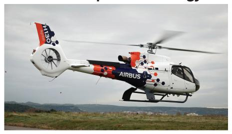
Airbus Helicopters recently introduced Flightlab, an agile and efficient test bed to test technologies that could equip Airbus current helicopter range. The Flightlab demonstrator will be used to test the hybrid and electric propulsion technologies and similar such technologies which will reduce helicopter sound levels, improve main-
