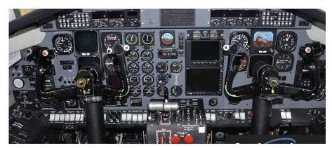
Southeast Aerospace (SEA) recently completed a major cockpit avionics modernization program on a SA 227 Metroliner. As a part of this process, they removed equipment including an early generation EFIS, many electromechanical and pneumatic instruments, and older communication and navigation equipment. Through the use of five STCs and
