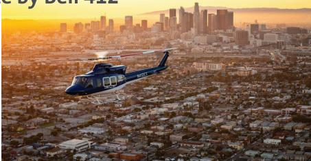
has been certified to run without oil (run dry) for up to 30 minutes for improved safety along with other evolutionary features.
