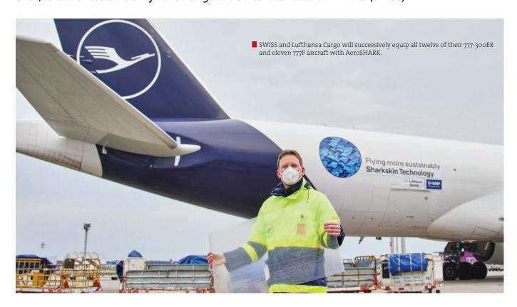
Lifthansa Technik and BASF have received a so-called Supplemental Type Certificate (STC) from the European Union Aviation Safety Agency (EASA) for the series modification of two Boeing 777 aircraft with the fuel-saving AeroSHARK riblet films. After being awarded the STC approval, the subfleet-wide roll-out of this sustainability technology which is developed jointly by Lufthansa Technik and BASF can now
