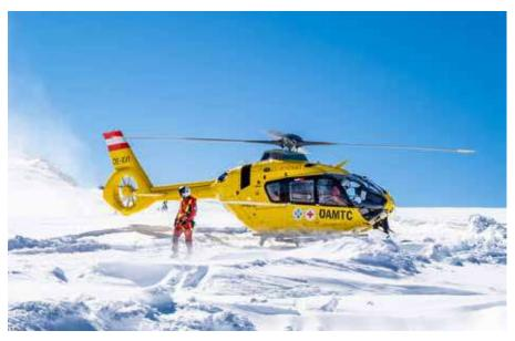
The H135 is the helicopter of reference for helicopter emergency medical service operators worldwide. It combines a wide, unobstructed cabin with excellent performance, range and payload capacity – along with low sound levels. The oversized sliding side doors and rear clamshell doors enable fast loading/unloading of patients, with additional safety during ground operations provided by Airbus' signature shrouded Fenestron tail rotor.
