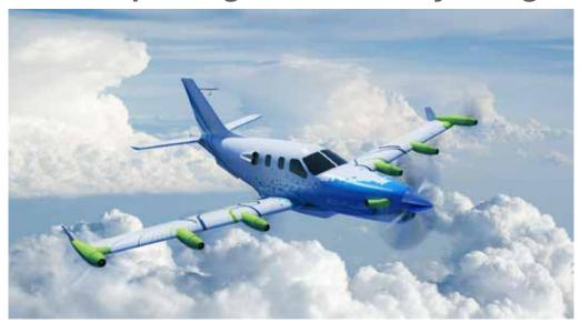
coPulse demonstrator has recently achieved its latest milestone with the passing of Preliminary Design Review, thereby paving a way towards the first flight scheduled for 2022. This has enabled the validation and freezing of the demonstrator's baseline configuration, as well as confirming the hybrid distributed propulsion system's level of safety and compatibility with the aircraft.
